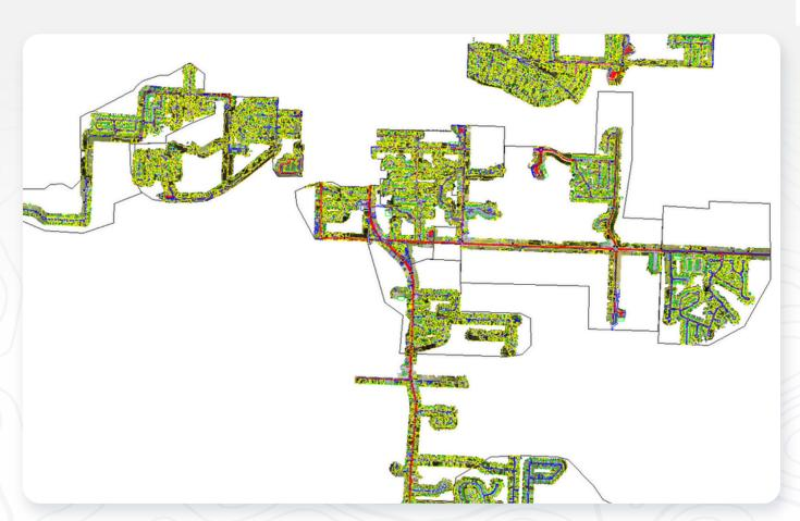
2D basemap with identified road centerlines, curbs, manholes, valves, handholes, catch basins, utility poles, and more to enable ROW and underground utility engineering in both high and low level design phases.
