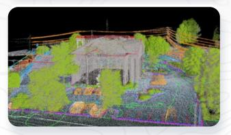
3D LiDAR point clouds used to create a digital twin of a project site, enabling measurement of distances, robust project site visualization, and accurate permit applications.
