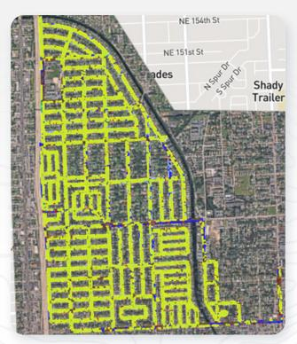
2D basemap with identified vegetation, roads, curbs, utility poles, pedestals, manholes, and more to enable ROW and underground utility engineering in both high and low level design phases.
