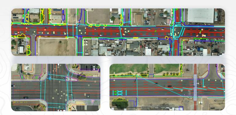
2D basemaps with identified pavement markings, utility lines, utility poles, vegetation, manholes, curbs, sidewalk, and more to enable strand mapping from UAV data of a project site
