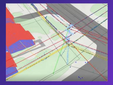
Utilizing the AirWorks software, a client can map and identify potential clearance violations via digital twin, working through an easily earmarked list of conflicts. This eliminates days of costly field work while improving the accuracy of these safety concerns.
